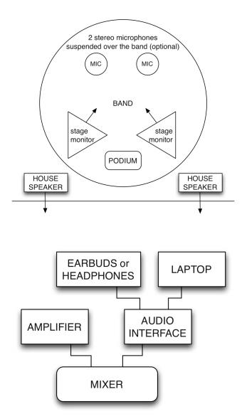
Monitors, speakers, laptop, audio interface, and microphones are connected by cables to the mixer, which is usually placed in the back of the auditorium or on the side of the stage. Additional technical information and suggestions may be found on the TIGHT SQUEEZE page at www.alexshapiro.org.
